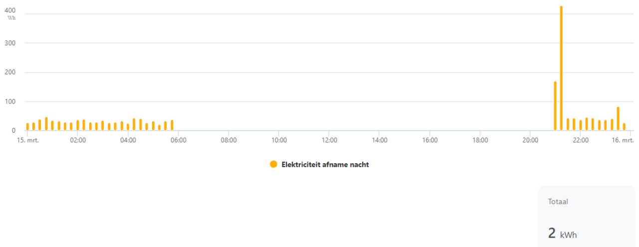
Figure 8: Electricity consumption of a household per 15 minutes measured by the night meter on 15 March 2023 [9]
